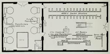
MAIN FLOOR PLAN, SUB-STATION C., SAN DIEGO CONSOLIDATED GAS AND ELECTRIC CO. Requa and Jackson, Architects
