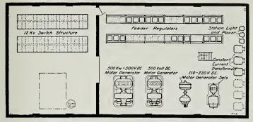
PLAN OF BASEMENT, SUB-STATION C., SAN DIEGO CONSOLIDATED GAS AND ELECTRIC CO. Requa and Jackson, Architects
