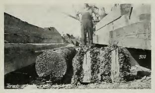
WHAT THE TEREDO ACCOMPLISHED IN TWO MONTHS AT CROCKETT, CAL. Wooden pile driven May, 1924, and pulled September 19, 1924. First attack of Teredo on July 15, Pile 12 inches in diameter completely riddled by Teredo at the mud-line shown in split sections. Courtesy of Prof. C. Derleth.
