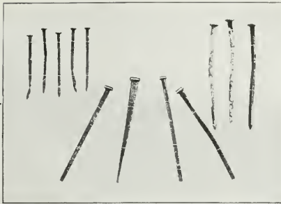
Copper-bearing steel nails driven in 1900 Wire nails of plain steel driven in 1900 Cut iron nails driven in 1886
