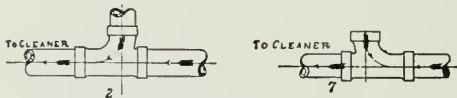
Always Place Y-branches So They Will Turn in the Direction of Flow
