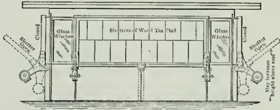
SMOKE VENT. MONITOR TYPE SIDE ELEVATION
