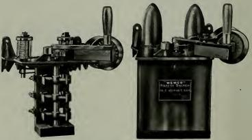
"Wemco" switches are used in the largest Industrial Plants on the Pacific Coast. They are equipped with overload and low voltage release; they operate in oil and are not dependent upon fuses. They are equipped with circuit breaker, which may be locked at its rated amperage. Your motor protection is absolute.
