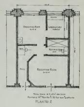
Getting the most of a space  $16'.8'' \times 23'.0''$  with two windows. Note the two operating rooms and the laboratory bench instead of laboratory room. Rental of 16 cents—§61.28 per month. The fallowing plans are all in a building with windows averaging 8'.4'' center to center, and with a distance of 23'.0'' from corridor to outer wall.
