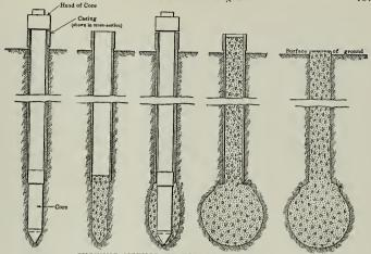
SHOWING METHOD OF FORMING PEDESTAL PILE
