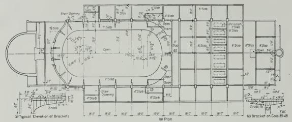
FIG. 3—CEILING OF SECOND STORY, ROOF OF TWO-STORY PORTION AND DETAILS OF BRACKETS SUPPORTING RUNNING TRACKS
