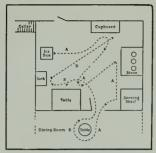
Floor plon of Applecroft Experiment Kitchen before it was arranged scientificolly. Note the confused network of steps resulting from inconvenient equipment wrougly placed. Preparing. b. Clearing away.
