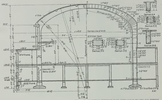
FIG. 1—CROSS SECTION THROUGH MAIN GYMNASIUM OF CHICAGO HEBREW INSTITUTE, SHOWING DETAILS OF ARCHES AND OF SUPPORTING COLUMNS Ottenheimer, Stern & Reichert, Architects L. I. Mensch, Engineer
