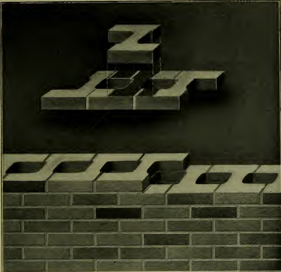
Fig. 1.—This new wall construction combines the mechanical advantages of concrete and the insulating properties of hollow tile, with the surface qualities of the best brickwork
