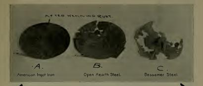
ERE is a photograph of results of what might be termed an Accelerated Exposure Test. Thin saucers made of American Ingot Iron, Open Hearth Steel and Bessemer Steel were all filled with cinders and set out doors for several months, at the end of which time they were found in the condition indicated.
