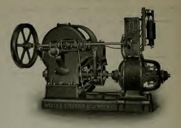
This plate shows a Direct-Electric Freight Elevator Machine, the type being instilled exclusively by the Spencer Elevator Company. The brake is cast in bloc with the gear casing, thereby making it rigid in every respect.
