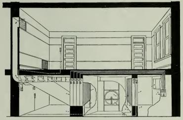
Plenum Hot Blast Heating System with Temperature Regulation
