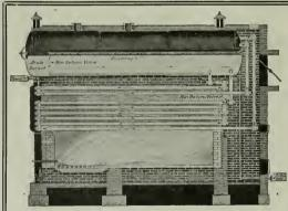
W1TH many tubes in one header, the unequal-expansion causes leaky joints. Rerolling thins the tube ends and means new tubes. In the design of a header holding but two tube ends each tube can expand without strain on header or joints. This is another feature of the
