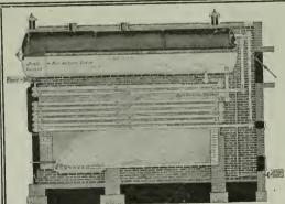
W1TH many tubes in one header, the unequal expansion causes leaky ioints. Rerolling thins the tube ends and means new tubes. In the design of a header holding but two tube ends each tube can expand without strain on header or joints. This is another leature of the
