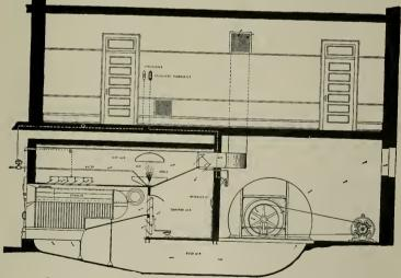
Furnoce Blast System of Heating with Temperature Regulation ond Humidity Control
