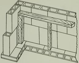
The above illustration shows a very successful method for supporting floors. These are as rigid as any wood construction can be. If desired tile can be substituted for the upright wood supports
