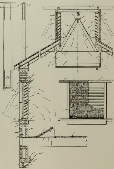
Fig. 3. Arrangement of Screens, etc., to Secure Desired Humidity, Showing Course of Air
