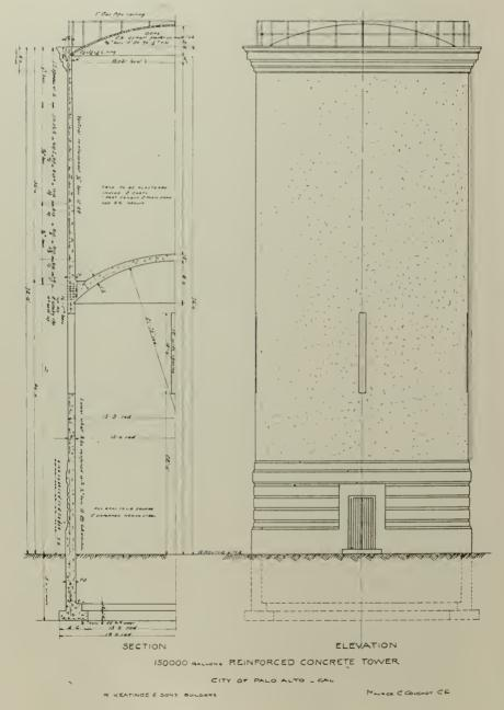
Sectional View and Elevation, Reinforced Concrete Tower, Palo Alto, California
