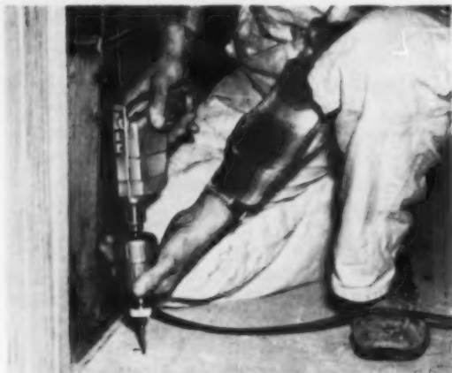
SLOWS UP THE SPEED —This Versamatic attachment fits a quarter-inch drill and slows down its speed. Result: it can drill concrete. At any ordinary speed the bit would burn up. Made by Supreme Products Corp. of Chicago.
