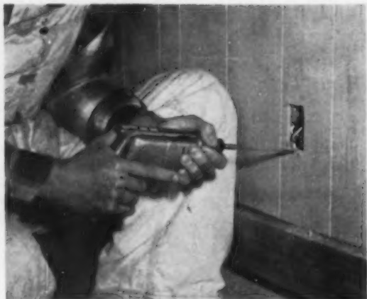
FITS ANY DRILL —Here's a Stickleback drill router that fits any quarter-inch drill. Used largely to cut outlet openings, it operates like a circular file. Can start hole, then drill opening. Tec Imports, Van Nuys, Calif.
