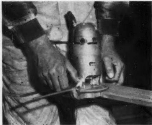
FOR ROLLING EDGES —This router has a molding bit attached to it. Purpose: to "roll" the edges of trim lumber or beams. Gives finishing a more decorative appearance. Also from Porter-Cable, Syracuse, N.Y.
