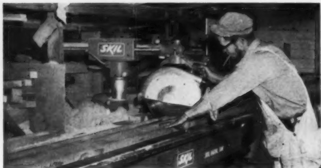
SAWYER WORKS outside assembly shed, has overhead weather protection. Cutting is done by radial arm saw—it's faster than hand saw.
