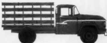
STAKE bodies from 7 \frac{1}{2} ' to 14' are built by Dodge on models to 19,500 lbs. G.V.W.
