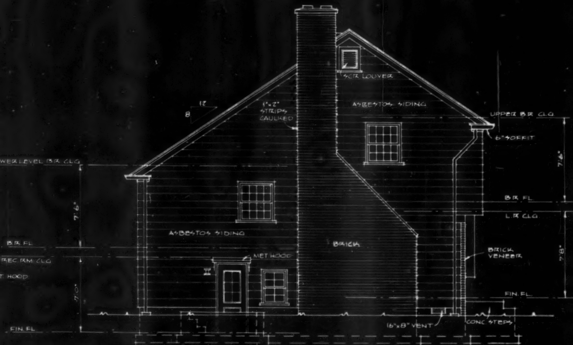
LEFT SIDE ELEVATION SCALE 1/8" = 1'-0"
