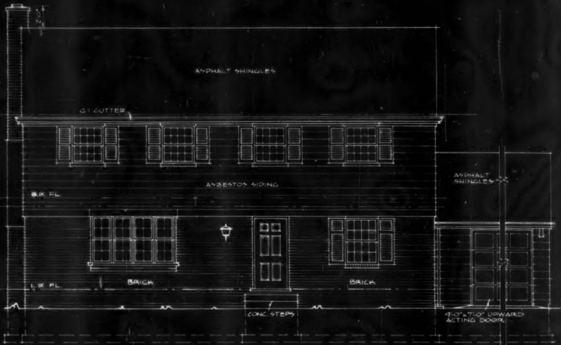
FRONT ELEVATION SCALE 1/8"=1'-0"
