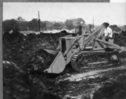
Bucket has a 35-degree roll-back at ground level for great "breakout" power.
