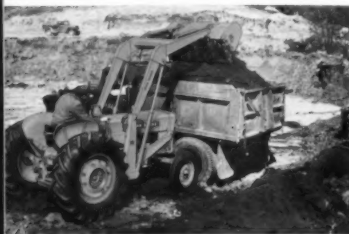
"440" Wheel Tractor with 71 Loader and 5/8-yard bucket does an efficient job of loading.
