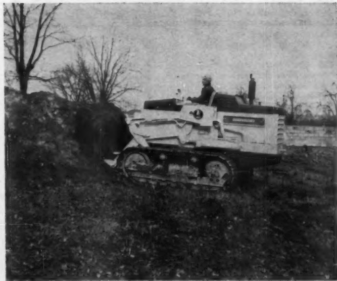
◀ CRAWLER VERSION OF THE "PAYLOADER" is the Hough Model 12. Treads give greater traction than tires, allow work in more difficult soil conditions. Note engine in the rear. Circle No. D73, page 106.
