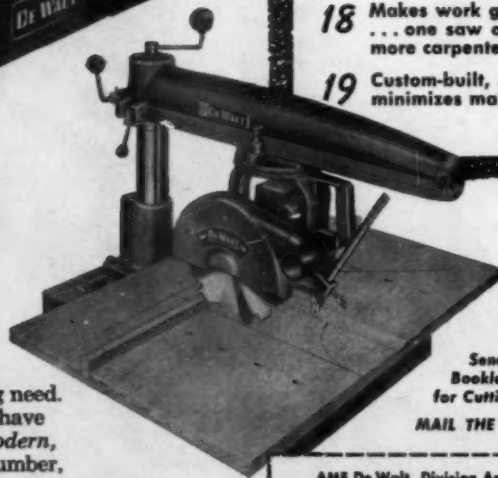
MODEL MB-F WITH 9" SAW. Portable, with new ¾ hp direct-drive motor, 120 V. 9" all-purpose saw blade cuts 2½" deep, rips 24" wide, cross-cuts 15" wide on 1" stock. Safety key switch, safety guard, and anti-kickback device. Weighs only 140 lbs.
