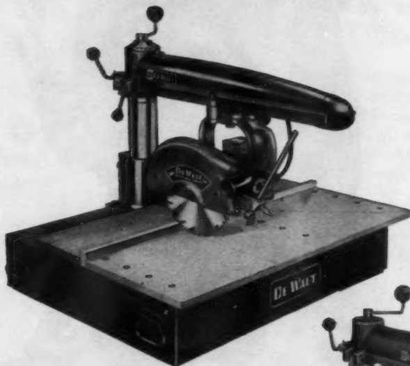
MODEL 6W-1 WITH 10" SAW. With 1½ hp direct-drive motor, 120/240 voltage change switch. 10" saw blade cuts 3" deep, rips 26" wide, cross-cuts 16" wide on 1" stock. Steel base with welded carrying handles, carries through 30" door. Safety key switch, guard, anti-kickback device. Weighs only 183 lbs.
