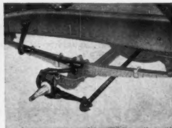
Shorter turning circles, safer and easier handling. Steering gears mounted ahead of the front axle.
