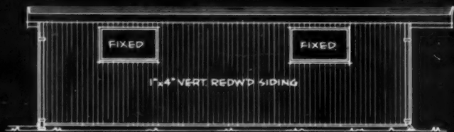
STORAGE - FRONT ELEVATION SCALE \frac{1}{8}'' = 1'-0''
