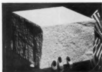
LIGHT IN WEIGHT , self-insulating and dry, with a "warm to the touch" feel—typical characteristics of a block of Elastizell-type concrete.
