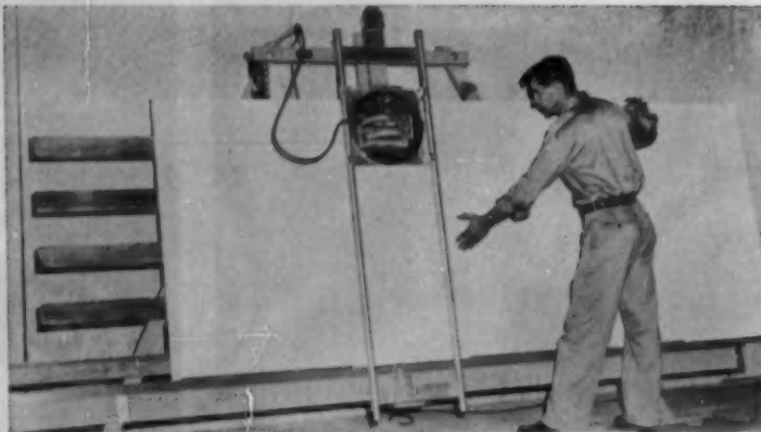
"TWO-WAY Panel Saw" eliminates wasted time, manpower, produces cleaner, more accurate cuts. It is 12 ft. long, 6 ft. 7 in. high, 24 in. wide. Weighs 140 lbs. One man can cut a
