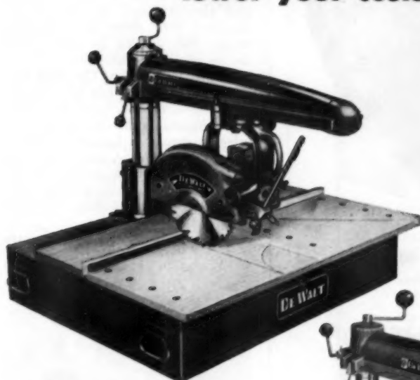
MODEL GW-1 WITH 10" SAW. With 1½ hp direct-drive motor, 120/240 voltage change switch. 10" saw blade cuts 3" deep, rips 26" wide, cross-cuts 16" wide on 1" stock. Steel base with welded carrying handles, carries through 30" door. Safety key switch, guard, anti-kickback device. Weighs only 183 lbs. $382.50 complete delivered.
