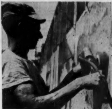
THE STOW RW wet-angle head for wet rubbing of concrete has an attachment for water hose so that water runs through center of grinding wheel. Button allows operator to apply water, grind at same time. The RW angle head can be connected to Stow's gasoline vibrators. List price: $70.62. Stow Manufacturing Co., Dept. AB, Attn. C. Hotchkiss, 443 State St., Binghamton, N. Y. Circle No. 1108 on Card, p. 188.
