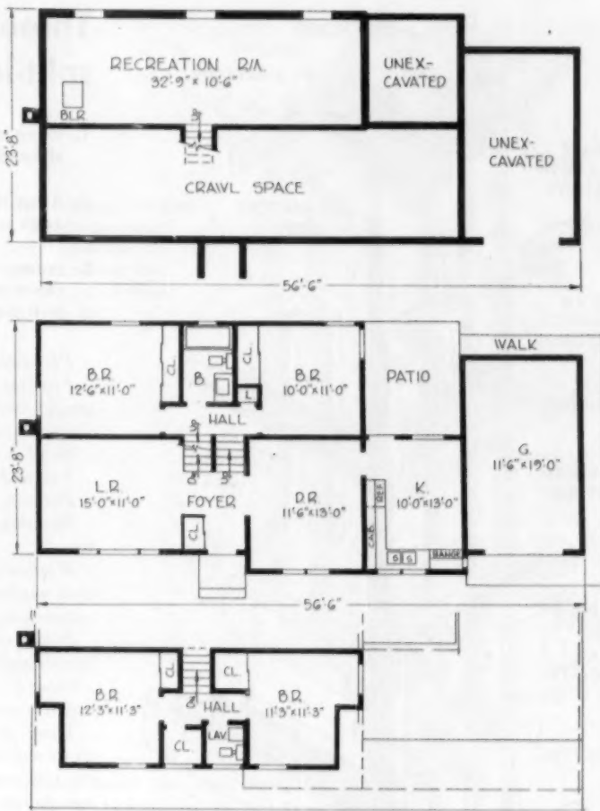
House plan is a simple rectangle with one bearing partition running entire length through center. This is also the line where change of level occurs, which simplifies framing.
