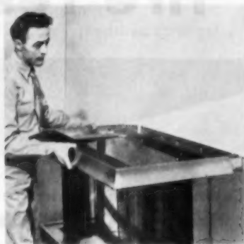
5. DOME TRIM is fastened to unit after flexible fire-screen is put in its place
