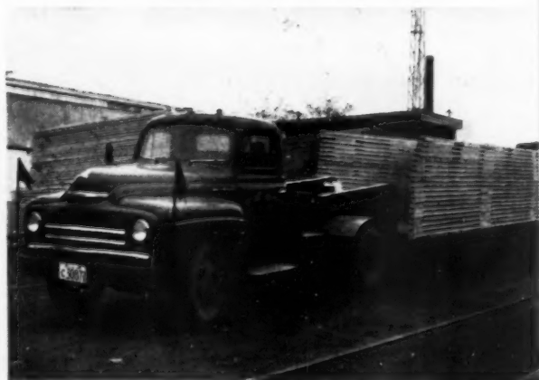
Finished panels or trusses are shipped via truck to the job site
