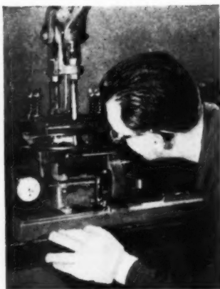
The ability of Kentile's top-grade raw materials to flow properly during calendaring is measured by a Mooney Viscometer .
