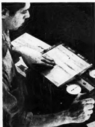
Trained technicians using Special Gauges check the length and width of Kentile to tolerances less than a thousandth of an inch.
