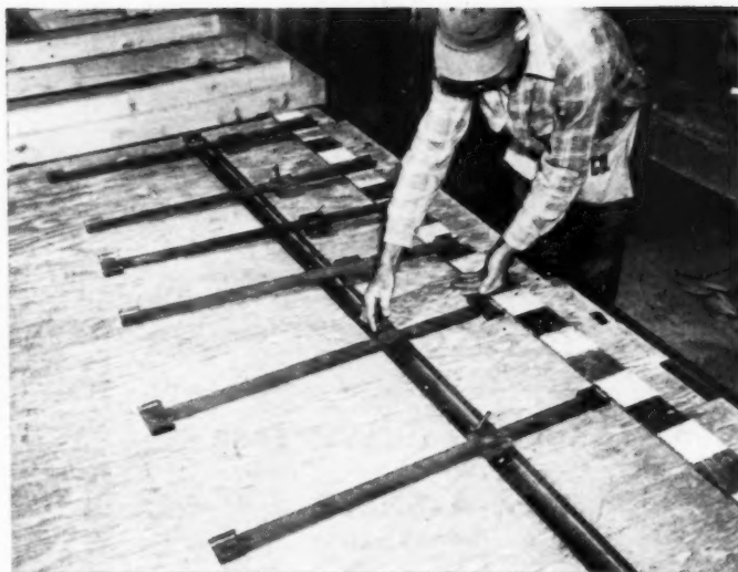
Step No. 1. Setting stud locators for rigid location of studs is quick, fast and easy
