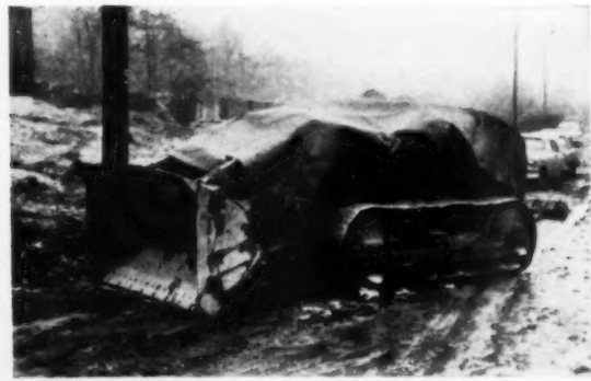
Cover your bulldozer in wet weather for easy starting
