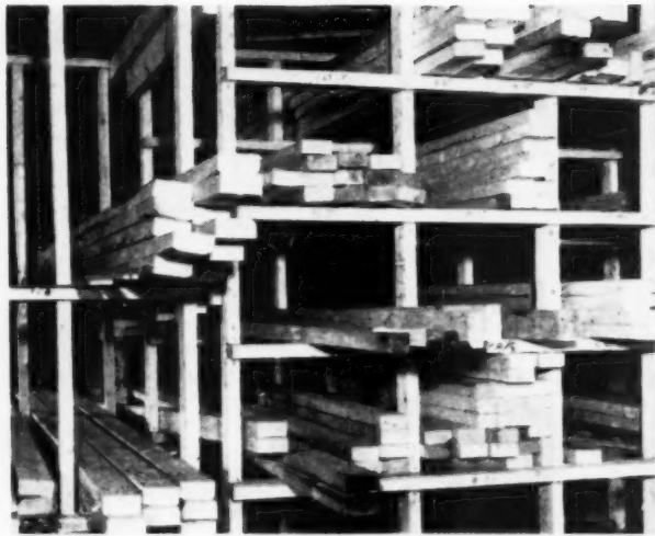
Material flows from yard through cutting bench (see below) to storage racks (shown above). Racks are located for easy access by assembly table workmen
