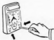
C Mount clock. Only four screws to fasten. Movement recesses into wall.
