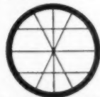
Fig. III—Special stadia hair arrangement, furnished upon request.
