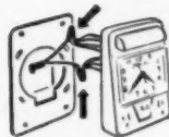
B Connect wires. Operates on 110 v., 60 cy. house current. Outlets rated at 15A.
