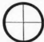
Fig. I—Cross hair arrangement for our standard levels.
