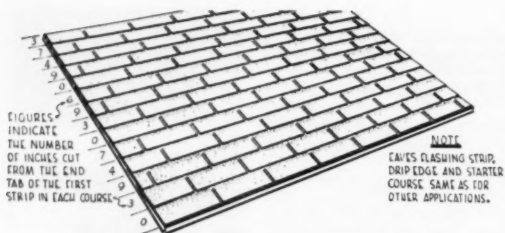
Random spacing of shingle tabs provides attractive appearance to roofs of one-story and one-and-one-half-story contemporary houses
