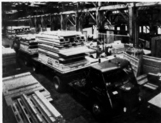
Wall and ceiling sections of two houses, one to three bedrooms in size, make up one load leaving the shop
