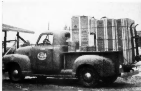
Heating-cooling system fits as packaged unit into light delivery truck. At left of unpacked equipment are steel blenders which give Blend-Air System its name
