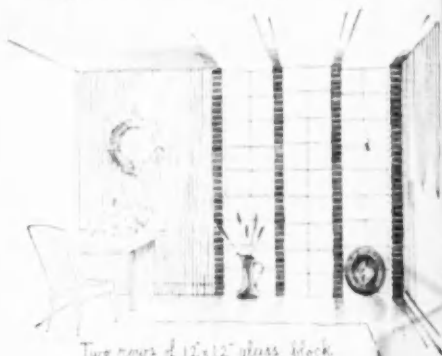
Two rows of 12x12 glass block in staggered plane with vertical brick fins.
