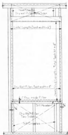
FIGURE 8. Framing detail of a typical rough opening for windows. Dotted lines outline different pieces of pre-cut dry wall sheathing
