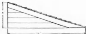
Pitch has a lot to do with the effectiveness of roofing. For asphalt shingles the pitch should not be less than 4 in 12
