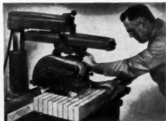
Big capacity . . . saw will cross-cut 25" wide on 1" stock, 22" wide on 5" stock . . . will rip to center of 77" wide panel.
