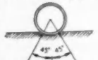
Bottom of pipe section, including 45° Arc from center, should be in firm contact with solid ground.
