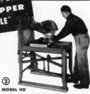
③ MODEL HD "CONVERTIBLE" CART used for SAWING CONCRETE
