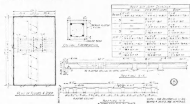
TYPICAL method of reinforced concrete joist (pan construction), beam and column framing, with integral fire-proofing
