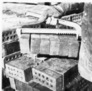
LIGHTWEIGHT tongs of magnesium contribute to easy handling of bricks
