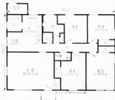
PLAN of the four bedroom home features bath-and-a-hall, dining area in the kitchen, and large wardrobe closets
