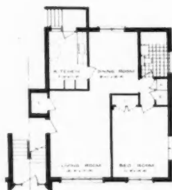
TYPICAL floor plans of Homestead apartments. Partition walls are not load-bearing
