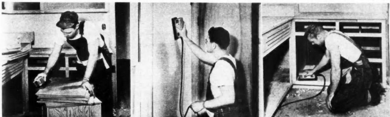
SHOWN at left is use of power hand sander in rounding and chamfering plywood edges. Power tool (center) takes place of hand method of sanding taped joint in dry wall construction. Right, note ease with which power sander is used in hard-to-reach areas
