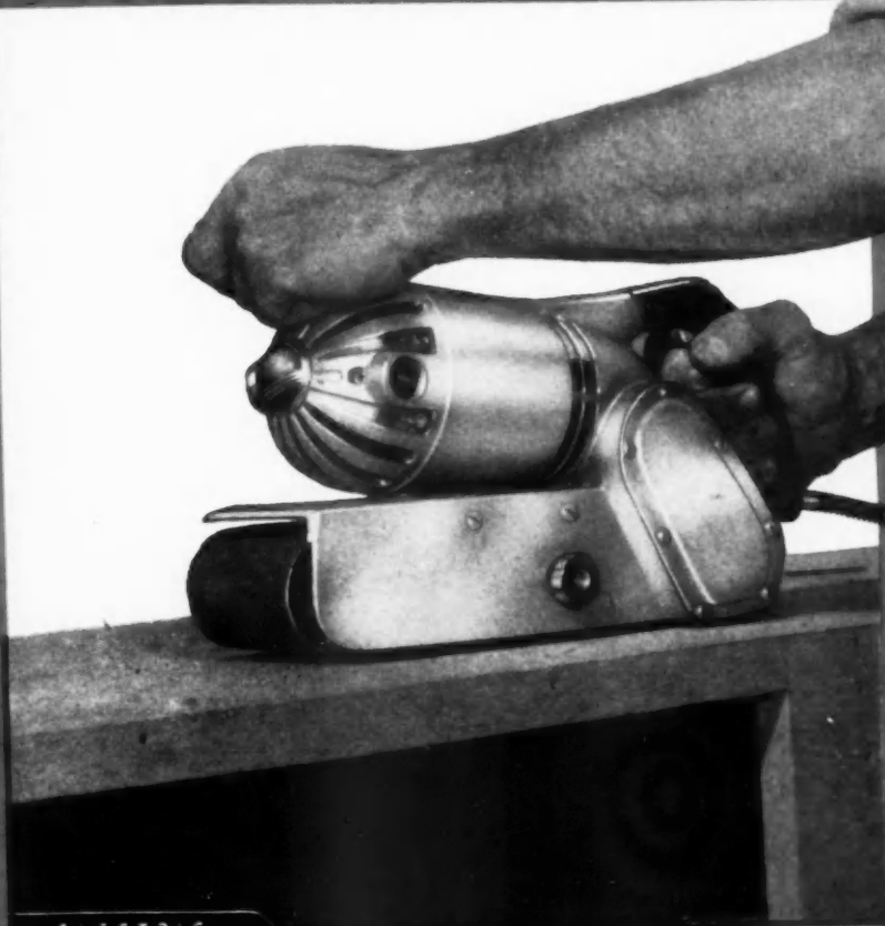
SKIL Belt Sander sands flat or contoured surfaces of all materials . . . wood, metals, stone, tile, concrete and compositions.
