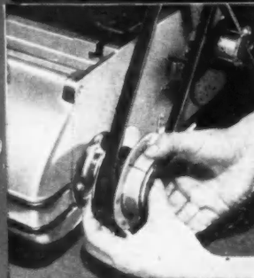
Special single adjustment pulley for speeds from 1600 to 2800 r.p.m. High speed position shown here—note small diameter of drum pulley.
