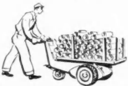
9-square-foot steel platform takes half-ton loads
