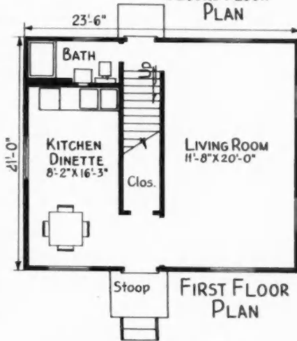
ARRANGEMENT of rooms in units. TEMPORARY exterior paper board covering with 960 square feet of floor area was replaced with fibre glass brick siding
