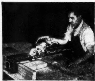
Saw Track No. 158 changes the Stanley Saw into a bench saw for production work.
