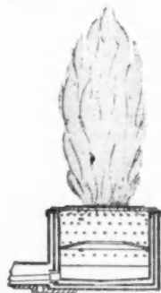
On high fire, flame leaves burner bowl entirely and burns above pilot ring.
