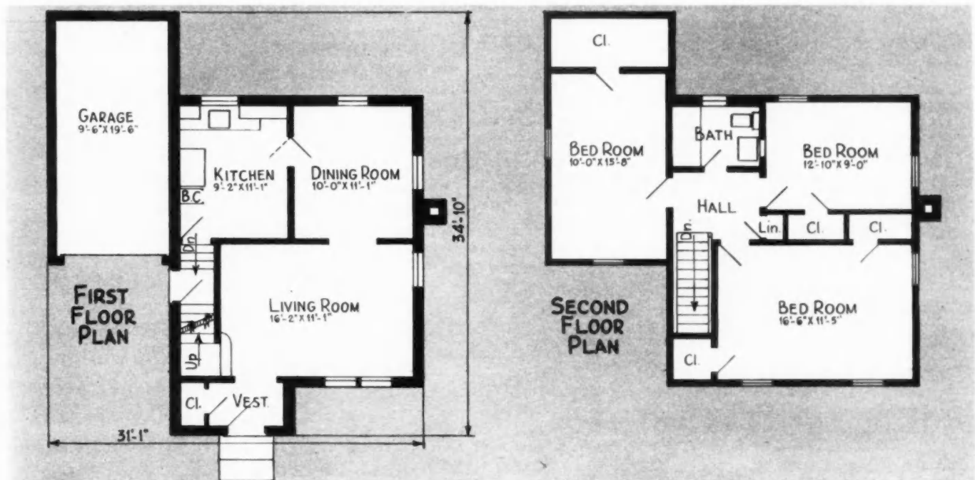
FLOOR PLANS for three-bedroom house. While rooms are not large, they are ample for modest living. The two-bedroom house floor plan is identical with this except that bedroom over the garage is eliminated.
