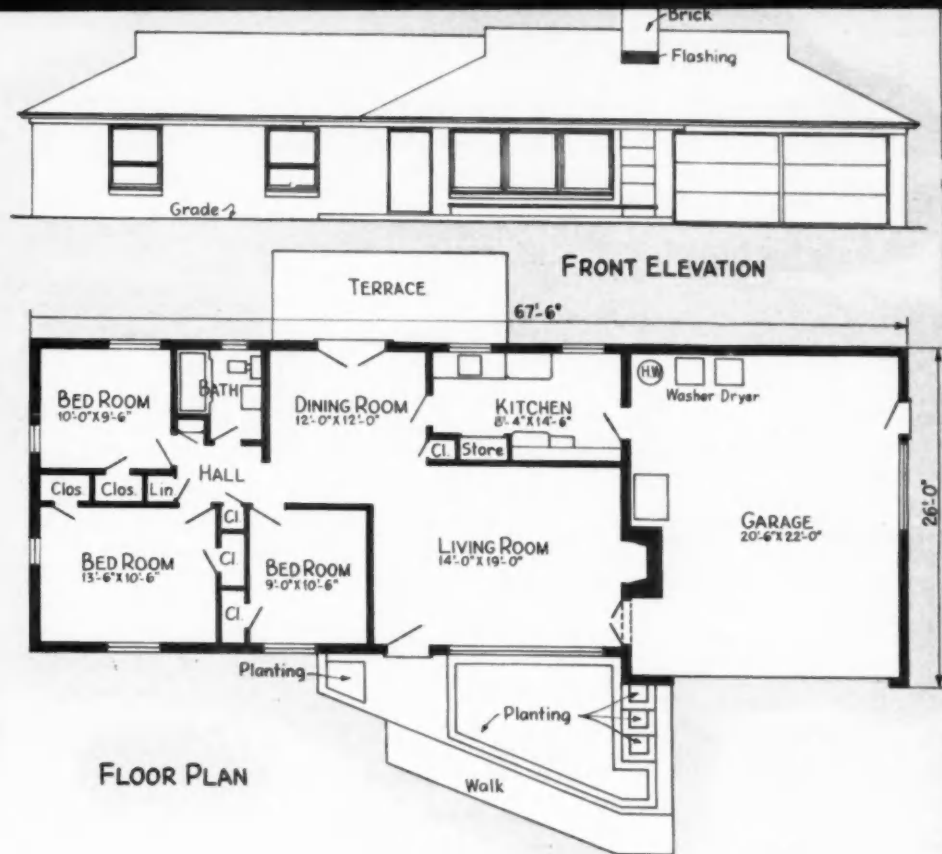
ABOVE is another of the popular floor plans and elevations for "Permatherm" homes.
