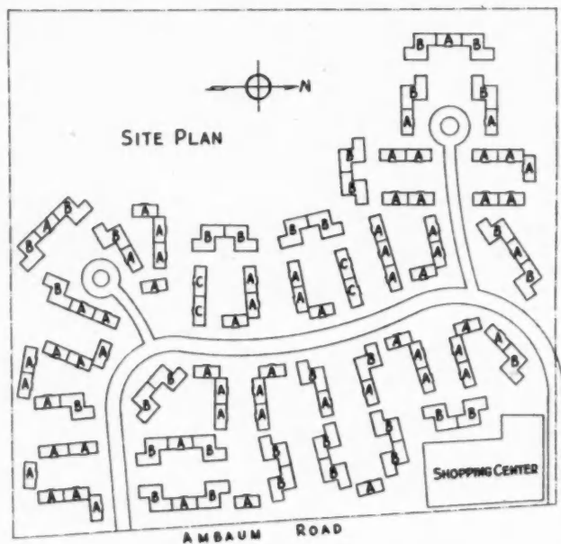
MORE than 200,000 cubic yards of earth had to be moved to level the site for 44 two-story apartment buildings and shopping center.
