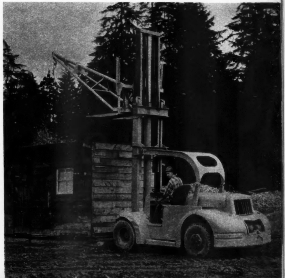
TOOL houses and work shanties are moved to new locations. With its 18-foot effective lifting range, bathtubs or other heavy materials may be hoisted to second-floor levels.
