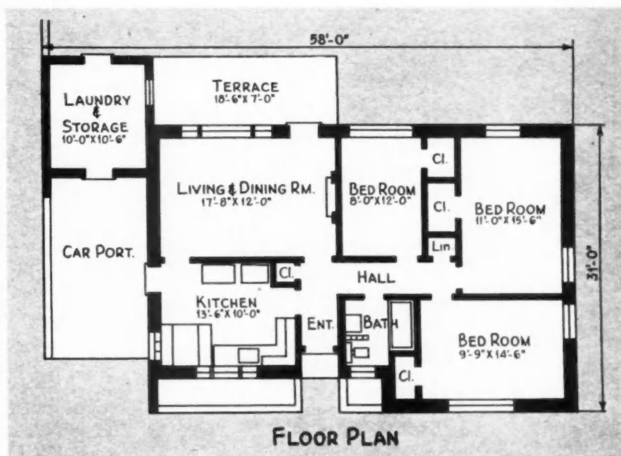
FLOOR plan of house pictured above shows three bedrooms, combination living-dining room, laundry and storage space.
