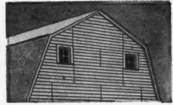
Weatherboard Siding. Sheets crimped like 4-in. clapboard. 8, 10, 12-ft. lengths; 24-in. coverage. Sturdy extra-thick sheet, .024-in.
