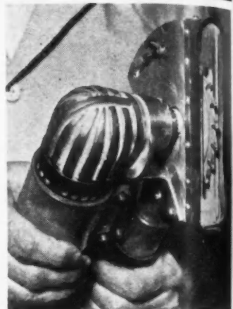
AB2630*—A new device which looks like an electric buzz saw attached to the end of a vacuum cleaner hose—and is—has been developed by Minneapolis-Honeywell Regulator Co., to simplify installation of personalized heating controls in existing buildings.
