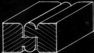
TONGUE & GROOVE REBATED. "D" MATCHED AND BEADED (M & B).
