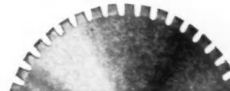
FRICTION BLADE for cutting corrugated, galvanized sheet.
