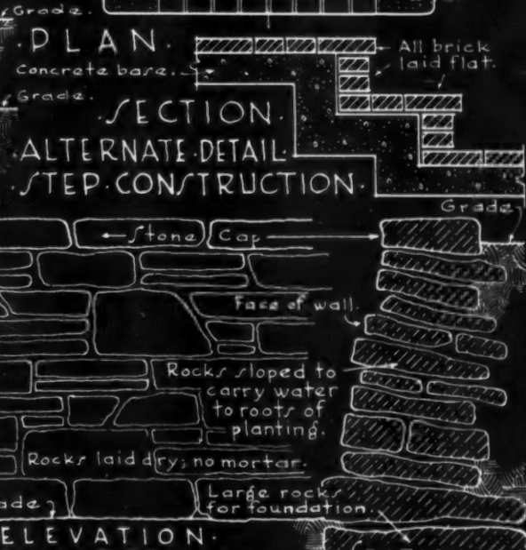
ROCK GARDEN WALL. ELEVATION. SECTION.
