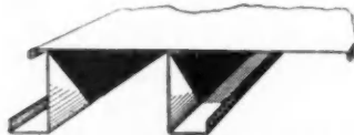
TYPE B. One flat surface and two channel-type ribs. Flat side up or down, inside or outside. 16" width, depth 3" to 9" elements of sections in combinations of 18 to 10 gage. As with Type A, permits easy application of wood, concrete or other materials for floors, walls or roofs.
