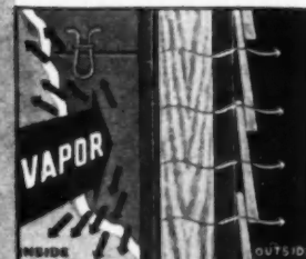
How moisture condensation is effectively minimized in the Approved Insulite Wall of Protection. Sealed Lok-Joint Lath, with asphalt barrier against the studs effectively retards vapor travel. Bildrite Sheathing, being permeable to vapor, permits what little vapor escapes to pass naturally towards the outside.
