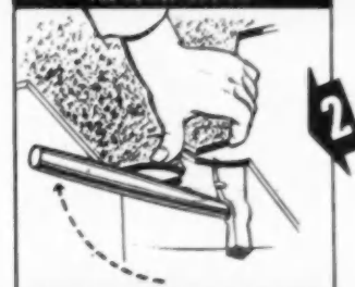
Insert locking slot of tab being laid with slot raised with the hatchet.
