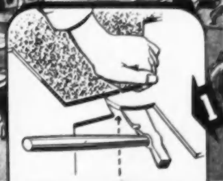
A twist of the hatchet lifts one side of the slot cut in the lower course.
