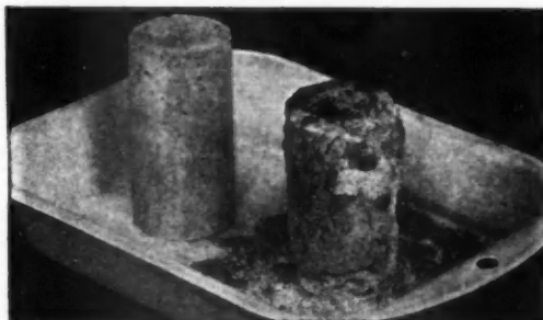
After curing for 30 days, 1/4" of water was put into the tray and the cylinders were alternately frozen and thawed 15 times. Note that the Brixment mortar remains intact, whereas the other mortar has crumbled badly.
