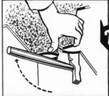
2 Insert locking slot of tab being laid with slot raised with the hatchet.
