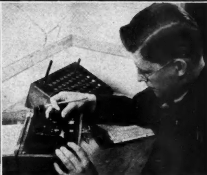
Taking Temperature Readings with Potentiometer at 43 Thermocouples.
