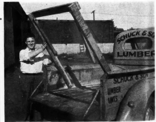
EXTENSION is swung up and out over end of truck bed. Note clearance at lower end of frame. Frank Kingery, one of Schuck & Son's senior employees, demonstrates rig which he helped design and build.
