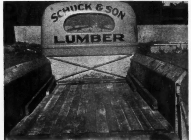
VIEW of truck body extension lying in truck bed when not in use. Note its compactness and small amount of room occupied within truck bed.
