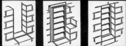
Leave opening in back wall Set ventilator in place Lay up front wall—and that's all.
