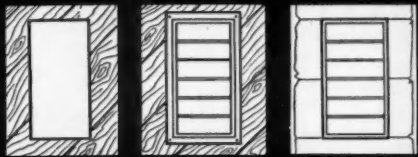
Cut opening in sheathing Nail ventilator in place Butt siding against body—and that's all
