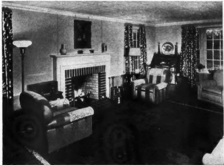
This room was ready for occupancy only a few days after the wiring was installed. The walls are built of Fir-TEX Colorkote panels and the ceiling of tile. When Fir-TEX is used, there is no waiting for plastering, plaster to dry, for wallpapering, or calcimining.
