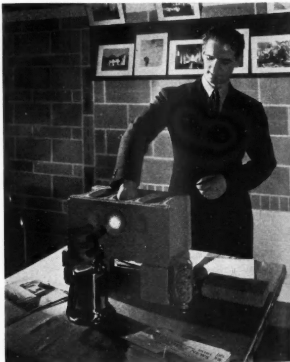
CONCRETE block of "Pottscoc" Lightweight Aggregate resists blow torch heat at Chicago Concrete Convention.
