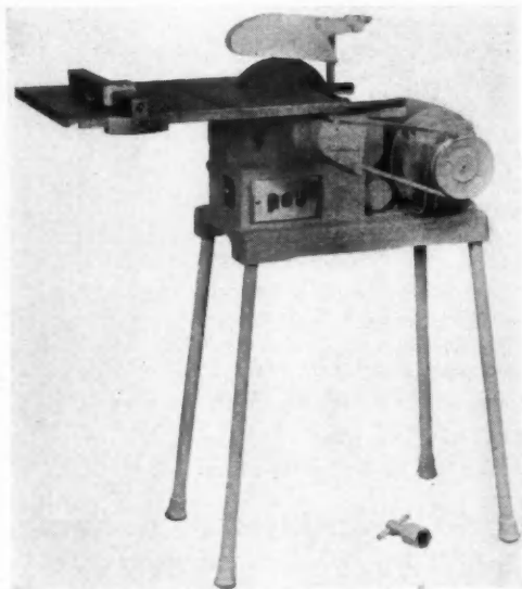
TILE and metal cutter can be handily carried on the job.
