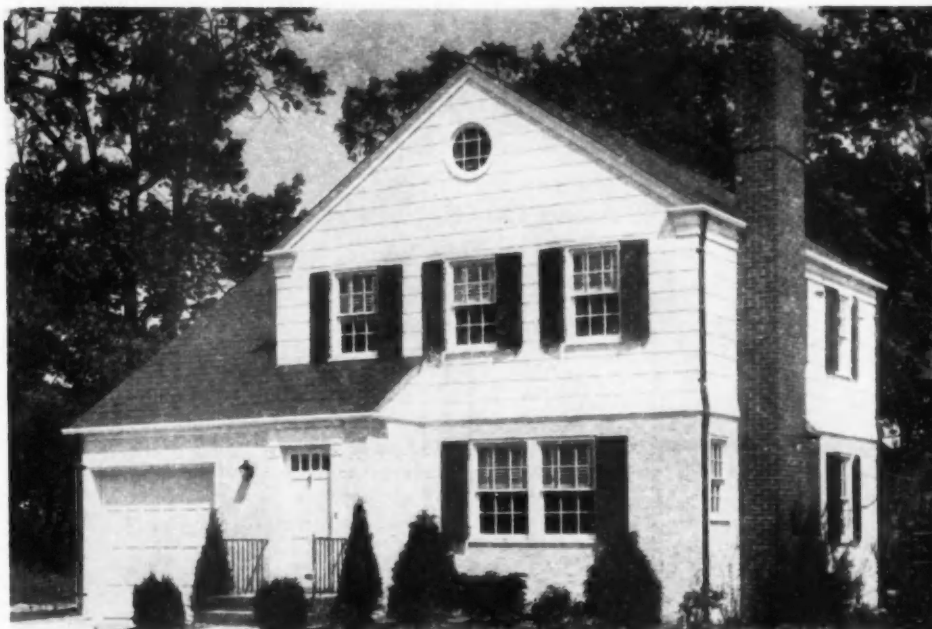
ONE of sixteen houses in the Loft Estates development on Long Island, the above design is typical of their good planning by Walter D. Spelman, architect. The six rooms and built-in garage are compactly arranged within an overall of 32'6" by 26'10". Numerous closets, breakfast room, well planned bath, cross ventilation and complete insulation of walls and ceilings with rock wool are features of this house.
