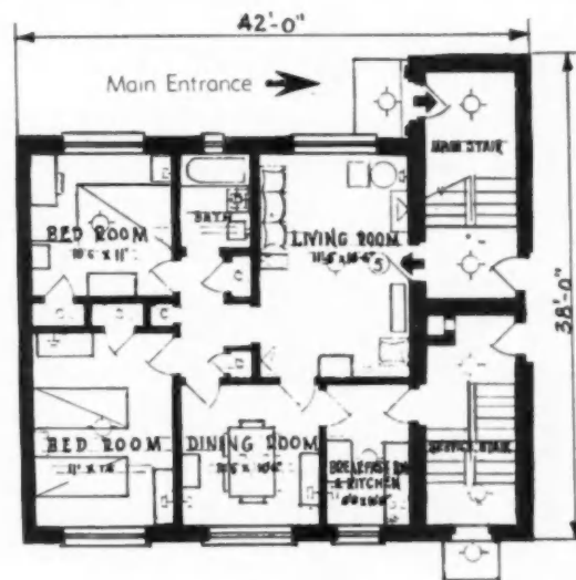
TYPICAL 5-ROOM APARTMENT floor plan located in buildings G-J-K. There are large windows. Living room is 11' 6" x 16' 6"; bath is located off convenient center hall. Kitchen has rear service door and stairs.
