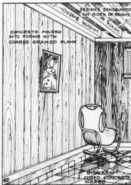
All-concrete room. Floor of Sisalcraft-cured concrete; walls of grained concrete; ceiling of sand-blasted pre-cast joist.
