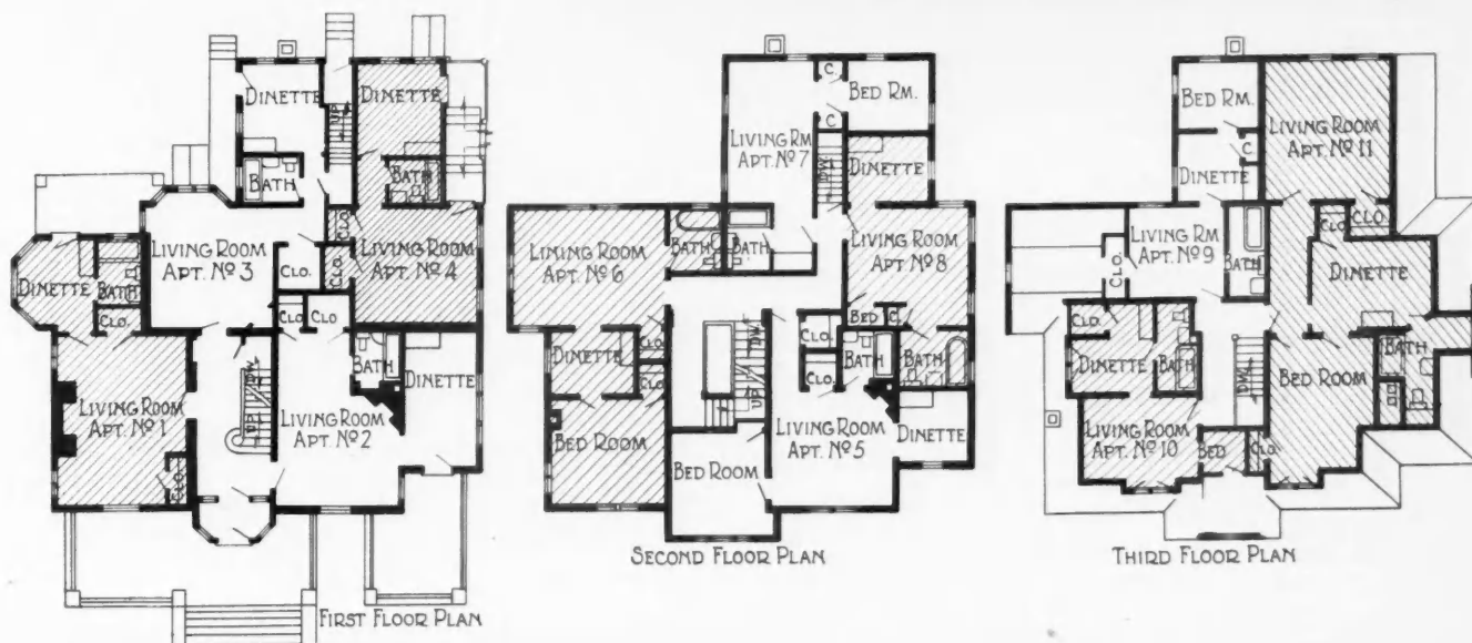
BELOW: Floor plans showing the layout of the units on the three floors with little structural change.
