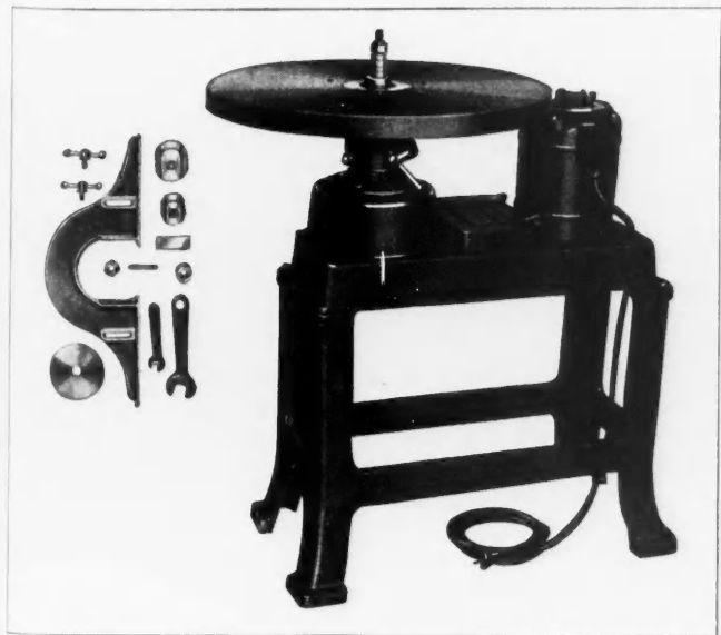
Spindle shaper with 24" cast iron table. Spindle is reversible; drive is new V belt type. Speeds of 6900, 8625, 10350 or 13800.
