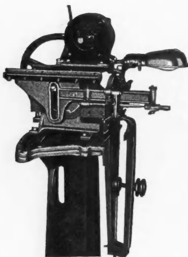
No Filings Can Reach the Bearing Surfaces.
