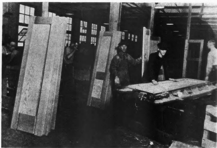
Here Is Seen the Assembly Work on the Doors After the Various Parts Have Been Built Up and as the Pins Are Placed for the Final Joining. After the joining parts have been coated with glue, they are given a squeeze in the powerful machine shown in the foreground.
