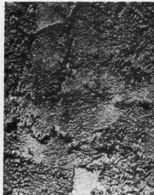
GOthic A float finish rough-torn with the back edge of the trowel
