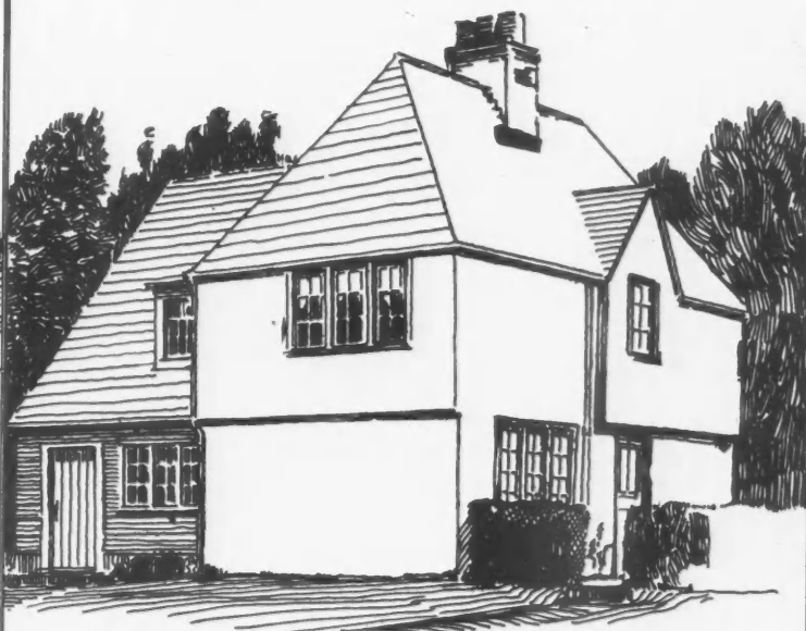
FIG. 2. THE HIPPED BLOCK WITH BLANKED WALLS
