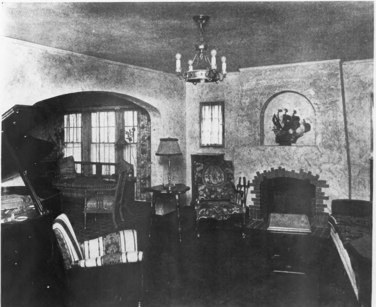
The Beautiful Living Room in the Residence of Mr. H. S. Ashenhurst. The walls and ceiling are rough cast finish over Gypsum Board.
