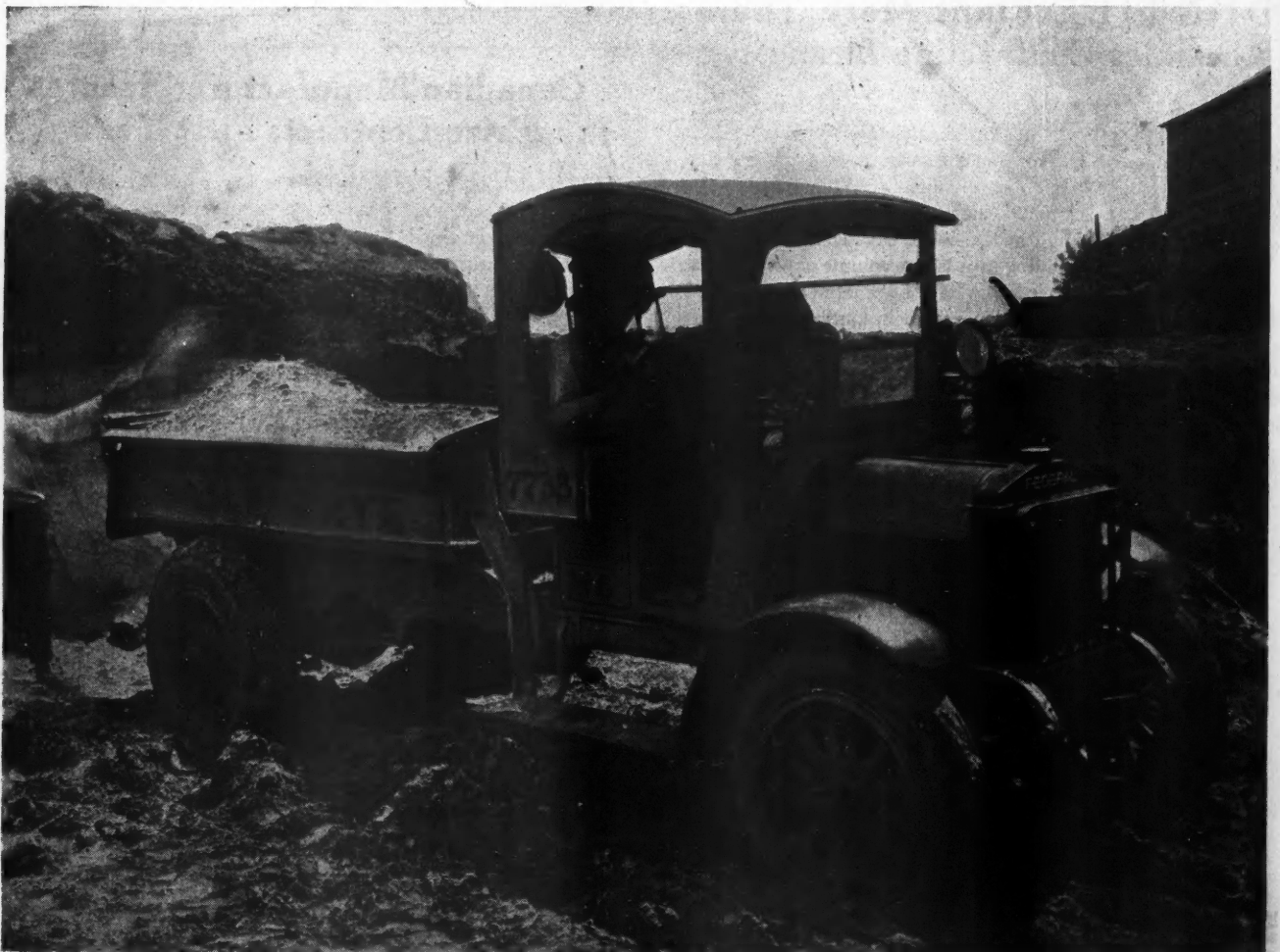
This Truck, Hauling Sand from the Pit, Was Carefully Selected for the Work It Was Expected to Do. It is a two-ton model with hydraulic hoist, dump body and pneumatic tires, which makes for quick unloading and good traction even in soft sand.
