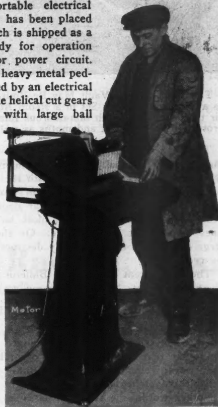
Shipped Ready for Connection to a Light or Power Circuit. This is a powerful, portable saw.
