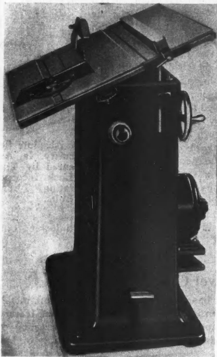
With This Machine One Man Is Able to Cut Long Stock Without the Aid of a Helper Because of the Swing Saw Feature.
