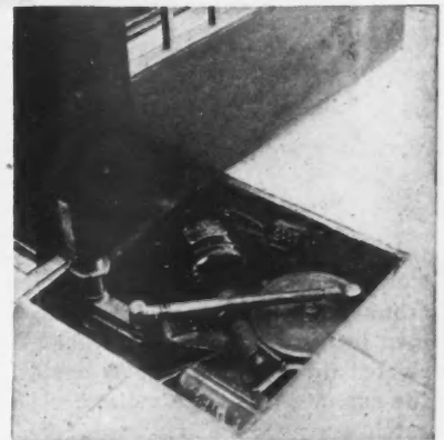
This Is the Little Device Which Will Open or Close the Heaviest Door or Gate Merely by Pressing a Button.
