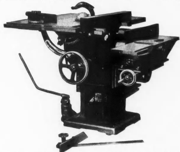
Most of the Builders' Woodworking Needs, on the Job, Will Be Taken Care of by This Portable Combination Woodworker Which Is Available at Low Cost and Is Easily Moved from Place to Place.
